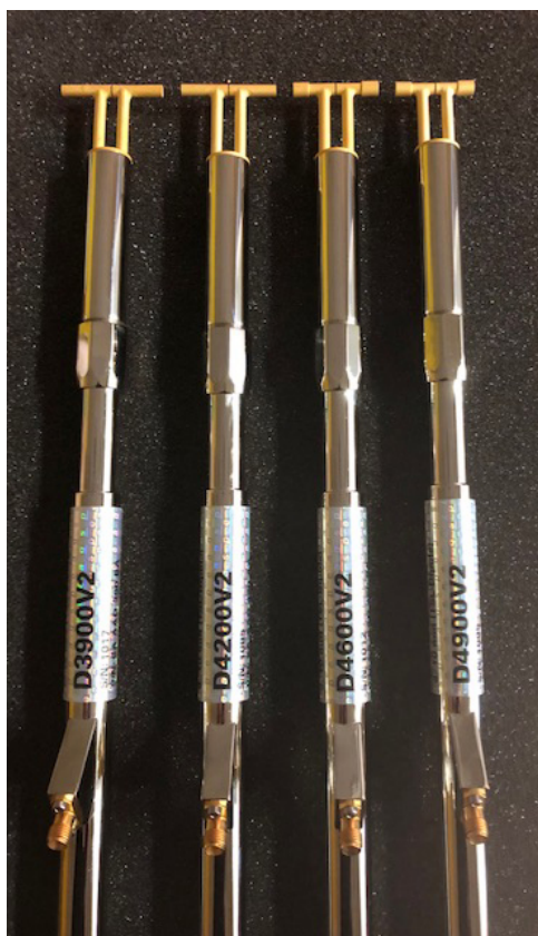
Figure 2: The 3900, 4200, 4600, and 4900 MHz dipoles, manufactured by SPEAG.
