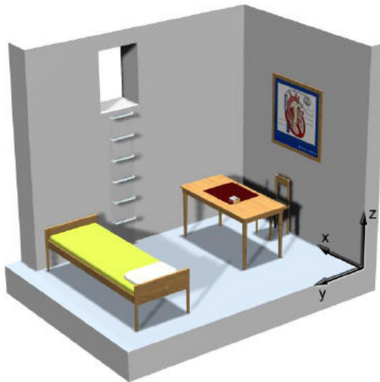
Figure 4 – CAD model of the simulated and measured “hospital room”.
