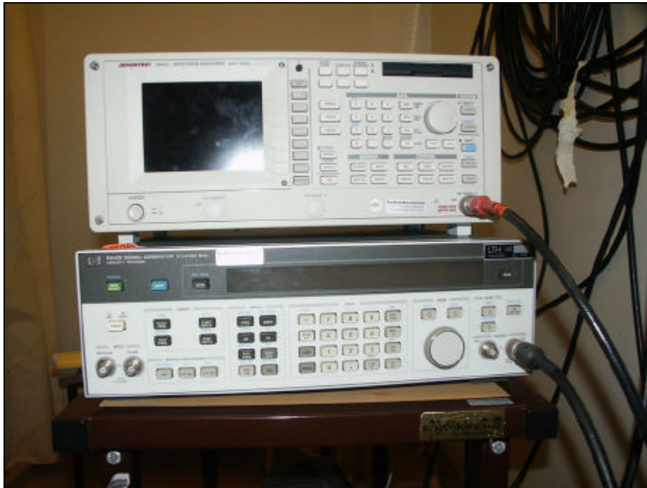
Photo 2 - The Advantest R3131 spectrum analyser placed above the HP 8642B signal generator.
