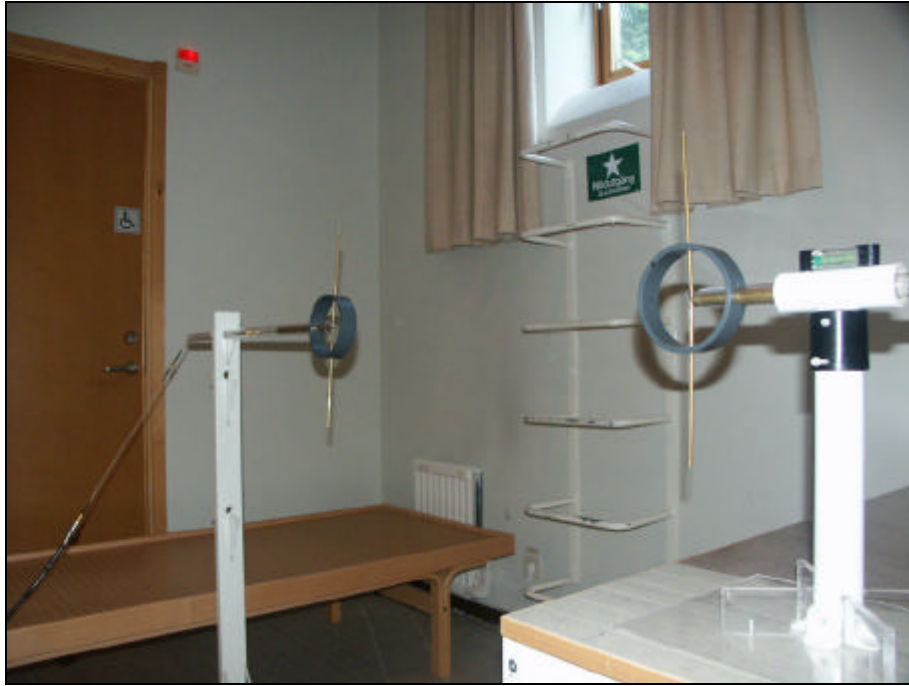
Photo 3 - Transmitting and receiving dipole antennas
